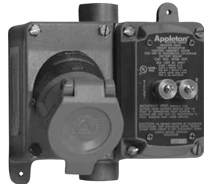
EFSR-GFI cover installed on two-gang EFD box together with U-Line 20A, 125VAC factory-sealed receptacle. Receptacle listed for Class I, Groups C and D, Class II, Groups F and G, and Class III.
