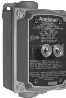
EFSR-GFI cover mounted on single-gang box. The GFI cover has separate factory-sealed sealing chamber and is suitable for Class I, Group B as well as Class I, Groups C and D; Class II, Groups E, F, G and Class III.
